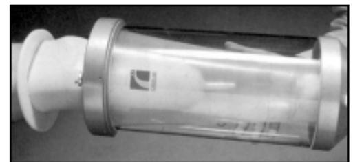
*ICECAST pressurized casting instrument used for creating TSB sockets.*
