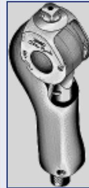
activated hydraulic knee. This new system provides a high degree of stance phase stability and cadence-responsive rotary hydraulic swing phase control. Its load-controlled hydraulic stance phase
