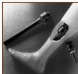
The **Stratus** can be used with standard modular components and various prosthetic foot designs. This pylon provides shock absorption by means of a compression ring, which can be ordered in one of five different degrees of cushioning to match amputee size and activity level. The Stratus pylon is rated for patients weighing up to 250 pounds and is said to reduce maximum force levels transmitted to the residual limb by 30 percent.
