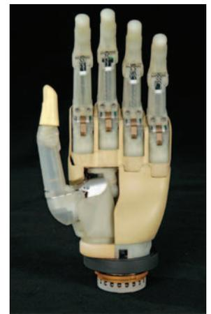
The i-LIMB is controlled by a highly intuitive control system employing a traditional two-input myoelectric signal to open and close the hand's life-like fingers. Myoelectric control utilizes electrical signals generated by the muscles in the patient's residual limb and picked up by electrodes on the skin surface. Existing users of basic myoelectric prosthetic hands adapt quickly to the system and can readily master the device's new functionality.
