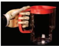
**Power Grip**—All the fingers and the thumb close down together to create a full-wrap grip, such as used to carry a can of soda or large objects such as a briefcase or shopping bag.
