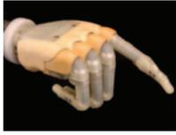
**Index Point**—The thumb and other fingers close while the index finger remains extended...useful for operating keyboards, a phone keypad, and controls on a steering wheel while driving.
