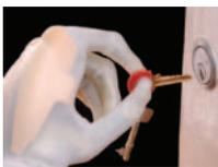
**Key Grip**—The thumb closes down onto the side of the index finger...used to hold items such as a plate or a business card...addition of wrist rotator enables the user to turn a key in a lock
