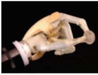
**Precision Grip**—The index finger and thumb meet, or the index finger, middle finger, and thumb meet to pick up and/or hold small objects when performing finer control tasks.
