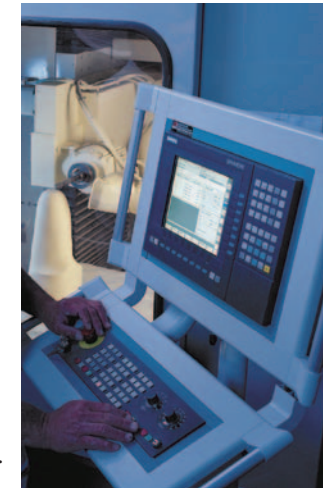
CAD/CAM carver brings digital precision to forming socket molds.
